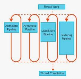
As we've stated before, for our purposes we're primarily looking at the Mali-T760. On the T760 ARM uses 2 ALU blocks per tri pipe, which is the most common configuration that you will see for Midgard. However ARM also has Midgard designs that have 1 ALU block or 4 ALU blocks per tri pipe, which is one of the reasons why seemingly similarly GPUs such as T760, T720, and T678 can look so similar and yet behave so differently.
